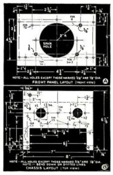
Fig. 4. Specifications of front panel and chassis.
